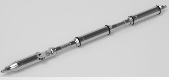
The ABM-40 is a MEMS based mapping tool specifically developed for generating accurate As-Built maps of duct segments up to 300m length. The standard ABM-40 has an outside diameter of just 36mm and is suitable for a pipe ID of 40mm (1.5"). Optionally, a spacer set is available to scale the unit incrementally up to pipes and ducts with an ID of maximum 75mm (3.0").
