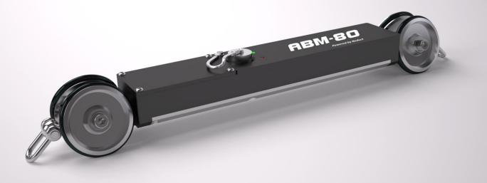
The ABM-80 is a MEMS-gyroscope based mapping tool specifically developed for generating accurate As-Built maps of short distance buried pipelines. The ABM-80 fits in pipes with an internal diameter of 80-500mm (3.2-20").
